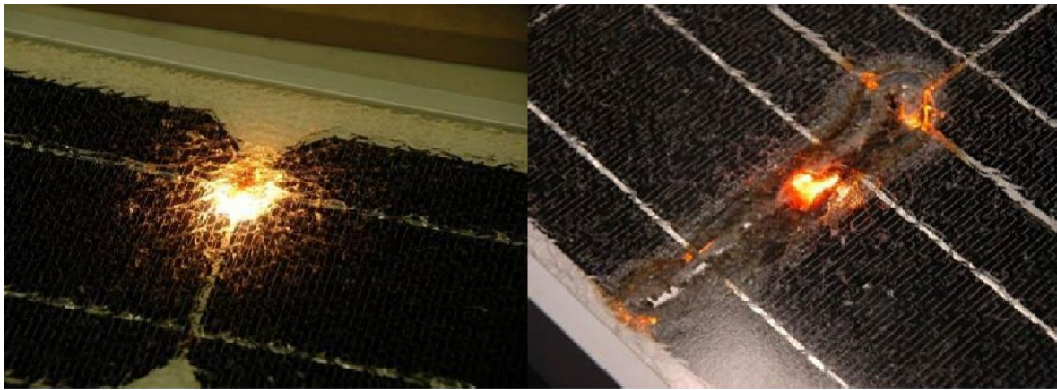
Image 2 Testing by TUV showing hot spotting within a solar panel caused by an electrical fault
