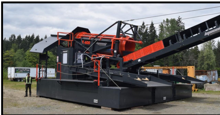
Fig. 7 – Indicative Floating Wash plant for Mining (Shown without the noise attenuating cover)
