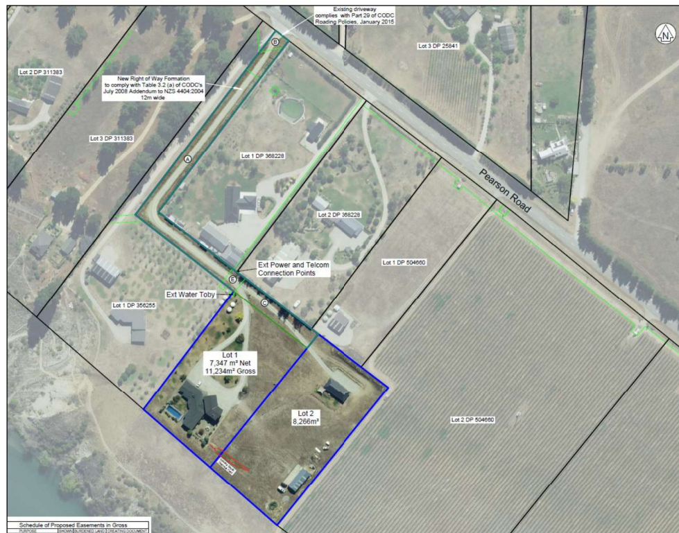
Figure 7: Extract of proposed scheme plan (Source: Latchford Surveying Ltd).
