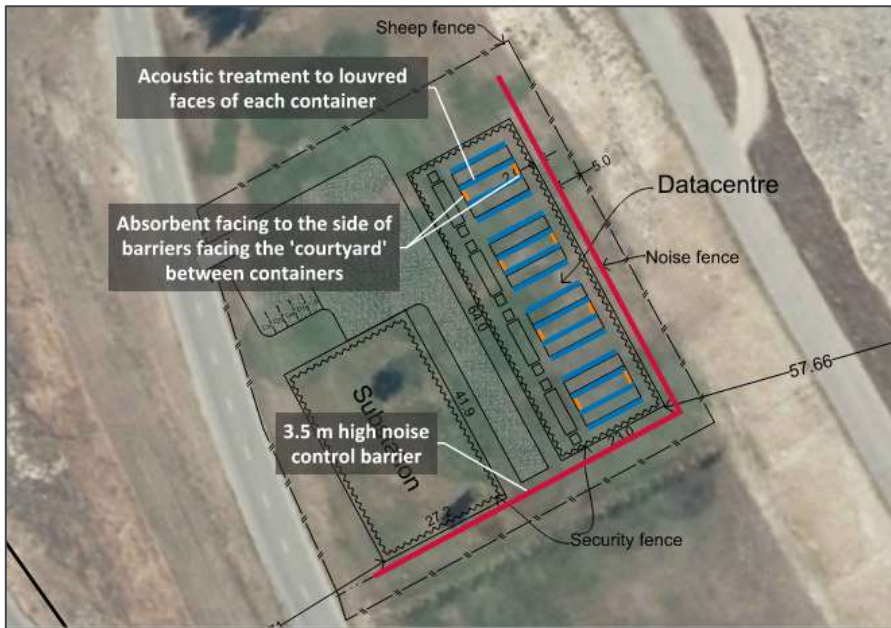
Figure 1: Location of noise control measures
