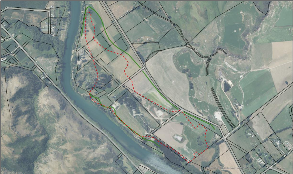
Figure 6: Bunding (shown by the green line) and extent of earthworks plan (shown in red). Source: Bunding plan dated 11 May 2023, titled Millers Flat Mine and completed by Town Planning Group.
