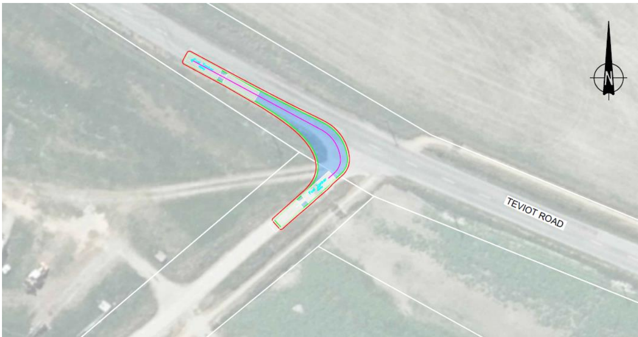
Figure 6.4 Left turn exit movement, southern access
