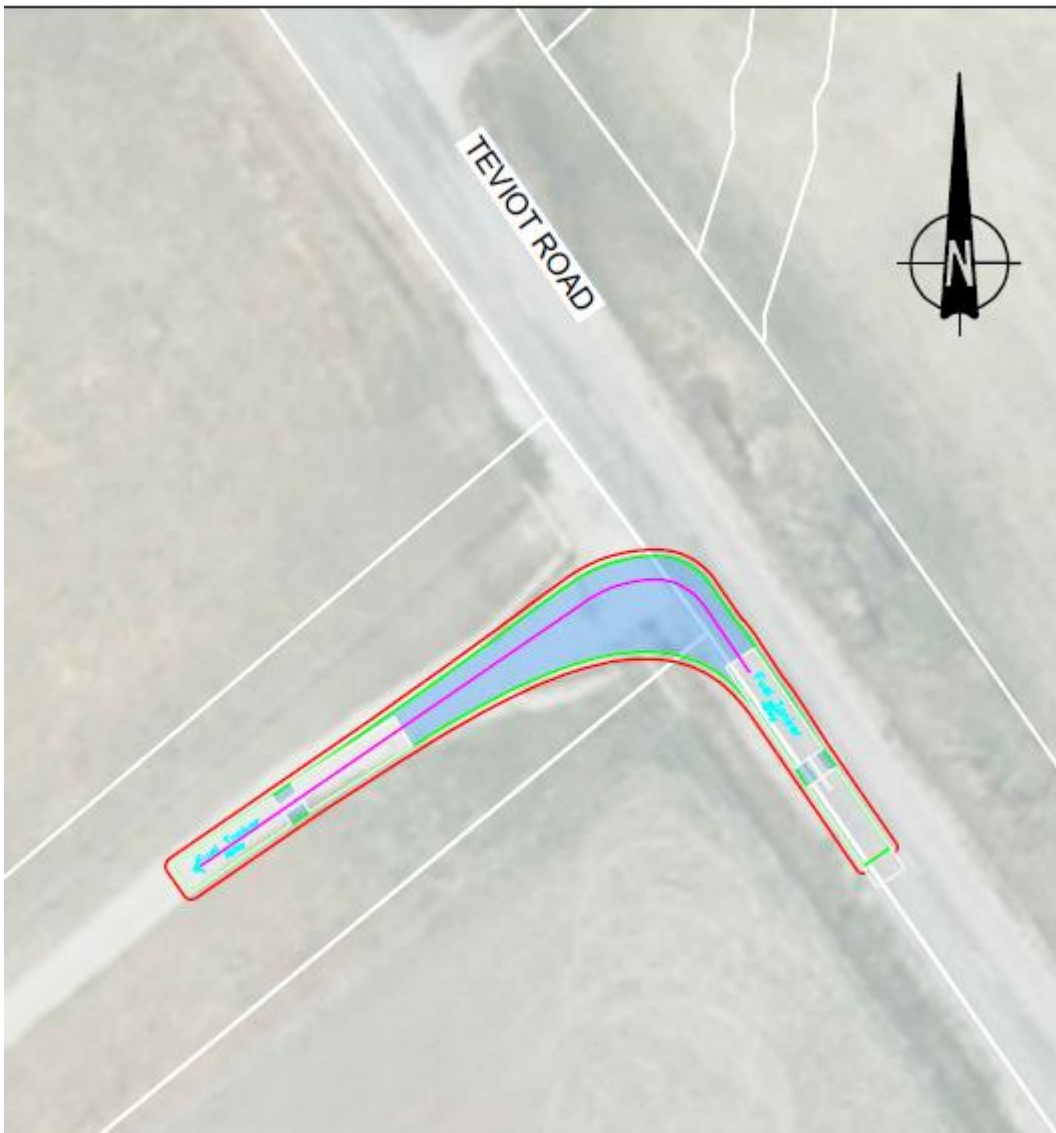
Figure 6.5 Left turn entry movement, northern access
