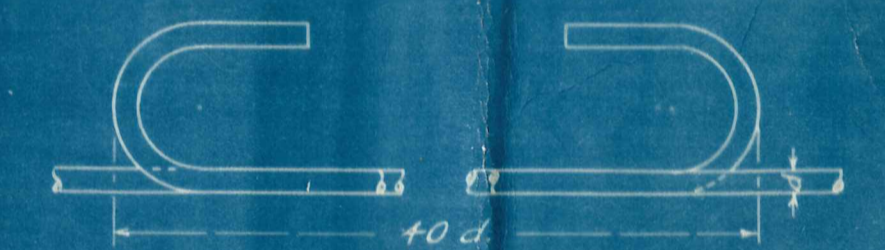
TYPICAL LAP JOINT NOT TO SCALE
