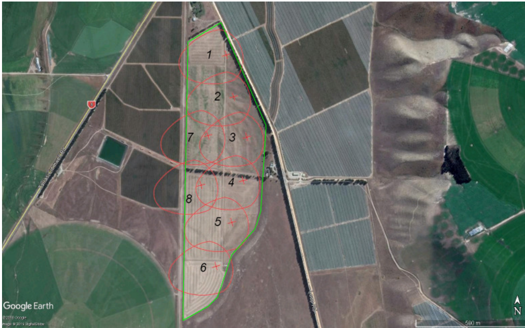
Figure 11b A comprehensive frost mitigation uses 8 wind machines. machines 7 and 8 provide significant overlap to machines 2 – 5, although a considerable portion of the warming footprint from machines 7 and 8 spill into the neighbouring vineyard.
