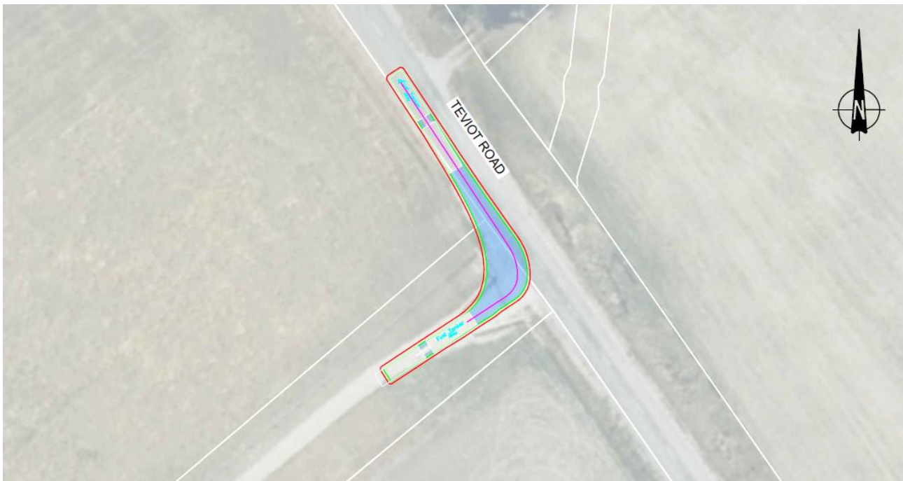
Figure 6.6 Left turn exit movement, northern access
