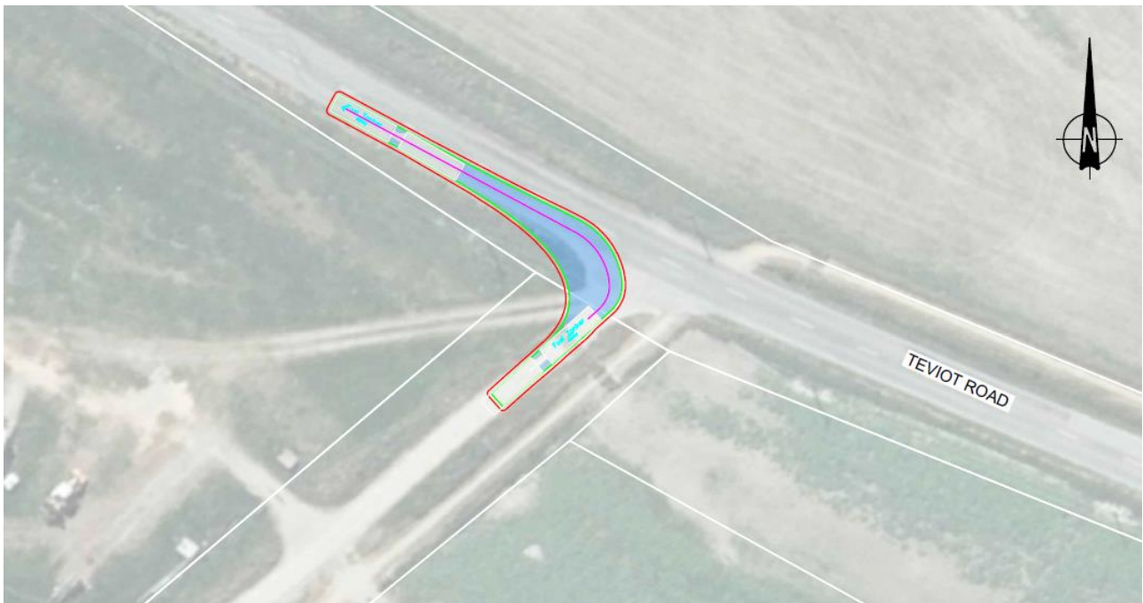
Figure 6.4 Left turn exit movement, southern access
