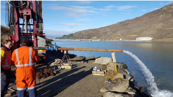
Three bores (including one new one) placed into the lake shore have now been proven to have the capacity to supply the area for at least the next 30 years.
